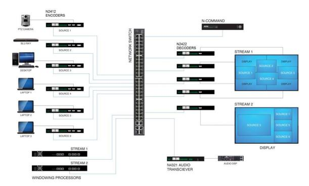
\*Note: Single line represents four independent connections from ports U0-U3 to the switch.
