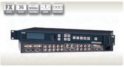
The ImagePRO-3G is a high-performance video scaler, scan converter, switcher, frame synchroniser and transcoder all rolled into one. ImagePRO is the ideal solution for converting RGB, HDTV, component, s-video, composite (NTSC, PAL and SECAM) and SD/HD/3G SDI video into a user-selectable video format. It includes four video outputs and three universal inputs, as well as a dedicated genlock BNC connector with loop-through.
