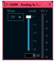
Click the Mute button to toggle the output's mute on or off, and drag the level fader to adjust the digital output level from -80 to 0 dBFS. The VU meter within the object will match the tool's horizontal VU meter associated with the output, and will reflect any changes made to the Mute or Level controls.
