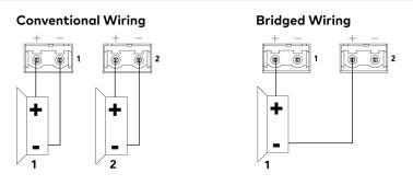
Speakers are bridged with the Crestron Avia® Audio tool, which can be downloaded from <u>www.crestron.com/software</u>. The possible bridging combinations are Output 1 & Output 2 (AMP-2800 and AMP-4600) or Output 3 & Output 4 (AMP-4600 only).
