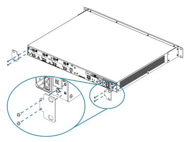
Then mount the device into the rack using four rack mounting screws (not included).
