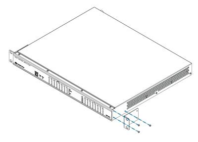
To install the included rear mounting brackets:
