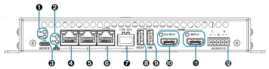
• OL and NV LEDs: Green OL LED indicates that the device is online with a control system.
