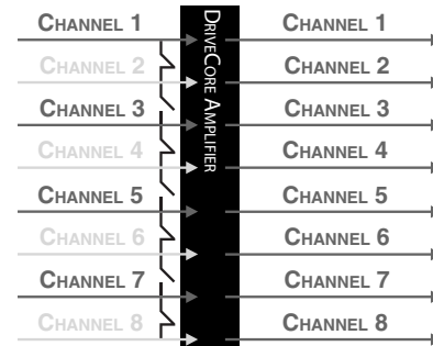
Figure 4.6.5 Four channel to eight channel routing
