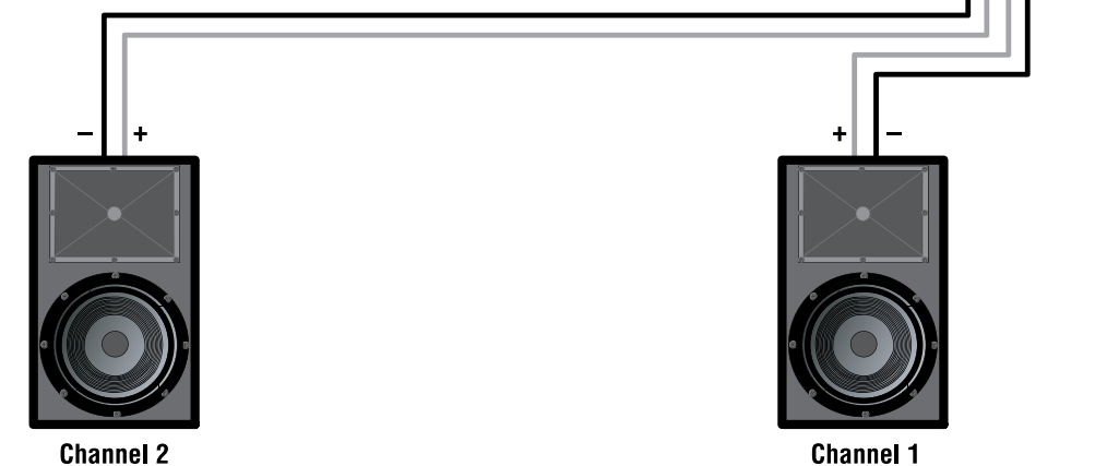
Figure 2.11 Stereo Wiring Using Both Speakon® Connectors
