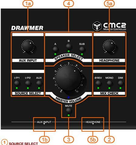
Thee switches select which of AUX (1b), I/P1 and I/P2 (6) inputs are heard at the Speaker Outputs (7) and Headphones (5). Each can be operated individually or simultaneously and in any combination. When operated simultaneously the individual signals are summed into a single stereo signal. Note that the CMC2 does not provide individual level trims for the I/P1 and I/P2 inputs and so any level matching should be applied before it reaches the CMC2.
