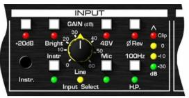
The preamplifier section is based around Drawmer's own discrete component mic preamp similar to that use in the well respected 1960, which provides very low distortion and a wide dynamic range with an equivalent input noise performance of -134dB.
