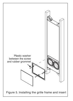
ful not to flatten the vibration isolating rubber grommets on the grille frame by overtightening the screws.
