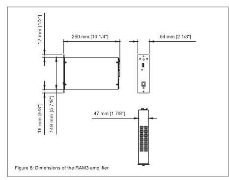
Sufficient cooling for the amplifier must be arranged at all times. As a general rule, the ambient temperature around the amplifier must not exceed 35 degrees Celsius ( $95^{\circ}$ F). The ventilation openings on the amplifier box must not be blocked and a free space of 1 U (=1.75" or 45 mm) must be left above the amplifier when installed. This space must be sufficiently ventilated to maintain the temperature below the maximum level.
