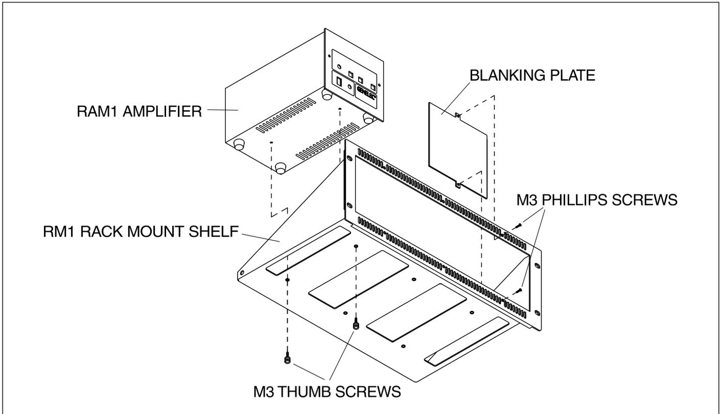
Genelec RM1 rack mount kit is custom-designed for Genelec RAM1 remote amplifier modules. The ventilation holes on the shelf plate and front panel of the RM1 match the location of the heatsinks on the RAM1 amplifier for maximum vertical air circulation and cooling effect. Because of this, three RAM1 amplifiers can be installed tightly together on a RM1 rack mount. If the ventilation holes on
