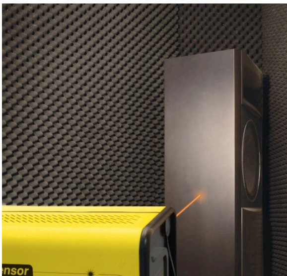
A laser interferometer can detect the source of resonance in a prototype enclosure
