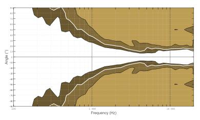
Dispersion angle diagram of one upright A10 Wide, using lines of equal sound pressure at -3 dB, -6 dB, -12 dB.
