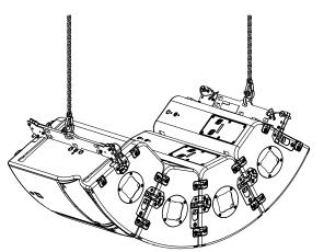
A10-RIGBAR can be used as the main lifting accessory, to provide a lightweight solution for flying four A10 Wide/Focus with one or two lifting points.
