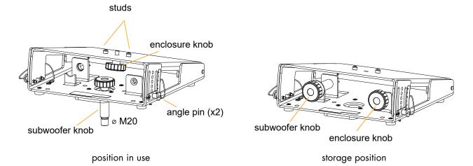
The opening angle of A-TILT can be adjusted between 12.5° and 25°.
