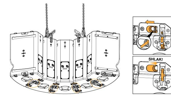
7. Lower the array to select the desired pickup points.
