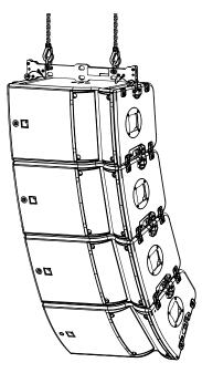
The pickup points are compatible with Ø12 mm shackles WLL 1 t (two provided) and CLAMP250.
