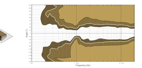
Dispersion angle diagram of one A10 Wide with 110° fins setting, using lines of equal sound pressure at -3 dB, -6 dB, -12 dB.
