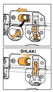
2. Secure A10-BUMP or A10-RIGBAR on top of the array.
