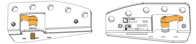
X-BAR is secured to the dedicated inserts on the enclosure, in front or rear extension position.
