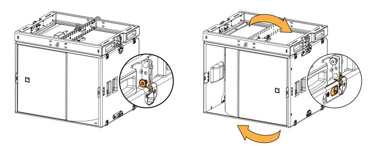
The rigging arms are fitted with yellow safety labels, that are visible when the rigging arm is not in use.
