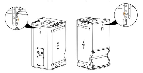
A DIN580-compatible M8 threaded insert is available to implement a secondary safety.
