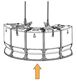
4. Disconnect the enclosures at the bottom.
