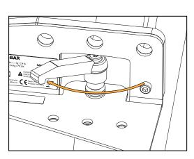
Repeat until the X-BAR is tightly secured.
