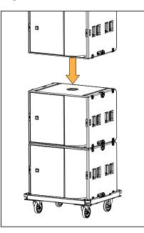
b) Connect the enclosures on both sides.
