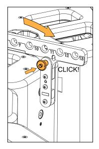
4. On each A10-LIFT, secure a shackle to the setup point (hole 8).
