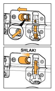
The rigging elements are fitted with yellow safety labels that are visible when they are not safely locked.
