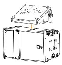
5. Secure A-TILT to the enclosure with the enclosure knob.
