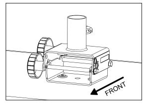
2. Remove the angle axis and secure A-MOUNT to the enclosure with the threaded knob.
