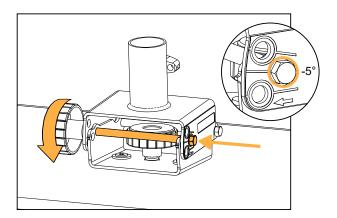
4. Mount the assembly on a pole and tighten the wedge clamp by hand.
