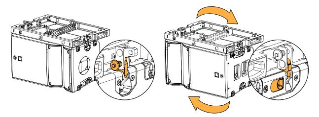
The rigging arms are fitted with yellow safety labels, that are visible when the rigging arm is not in use.
