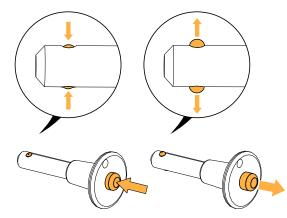
**3.** Insert the pin in each storage and rigging hole. Pull and rotate the pin. The pin must remain inside the hole.
