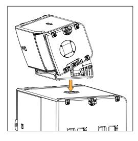
7. Adjust the position of A-TILT and secure the subwoofer knob inside the pole-mounting socket.
