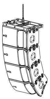
A10-BUMP can be secured to the bottom of the array to implement pullback configurations, using the rear pickup point (R). Alternatively, A10-RIGBAR (p.27) can be used for pullback.
