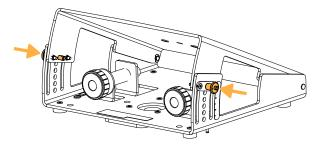
**4.** Place A-TILT on A10 Wide/Focus, using the locating pins for positioning. Consider the final position of the enclosure.
