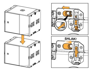
2. Secure A15-BUMP or A15-RIGBAR on top of the array.
