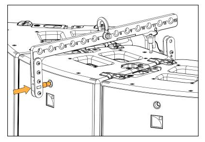
c) Insert the stub at the rear and secure the ball-locking pin.
