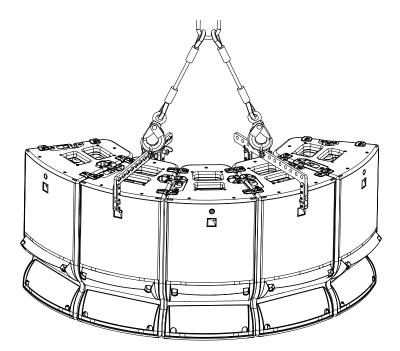
13 holes are available for site angle adjustment. They are compatible with Ø12 mm shackles WLL 1 t (two provided) and CLAMP250.
