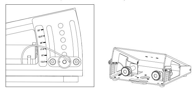
Four  $\emptyset$ 11 mm holes are available to secure the assembly to the floor.
