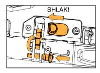
Connect A10-RIGBAR to the bottom enclosure on both sides.
