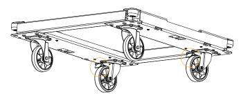
2. Place KS21 on KS21-CHARIOT and connect the two elements on both sides.
