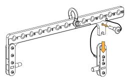
b) Insert the stub at the front of the enclosure.
