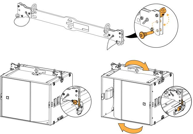
The rigging arms are fitted with yellow safety labels, that are visible when the rigging arm is not in use.
