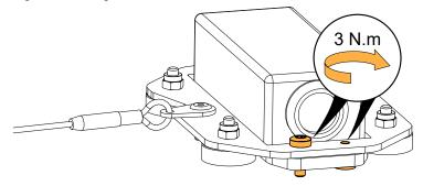
**4.** Place the LASER-MAGPLATE to the flying frame or to the enclosure.
