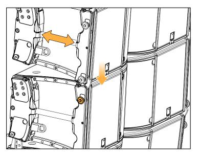
**2.** Lock the inter-enclosure angles of the block.
