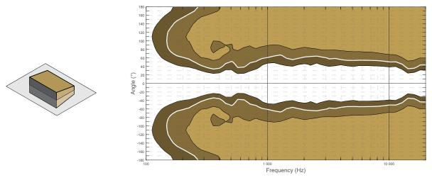
Dispersion angle diagram of a K3 array with 110° fins setting, using lines of equal sound pressure at -3 dB, -6 dB, -12 dB.
