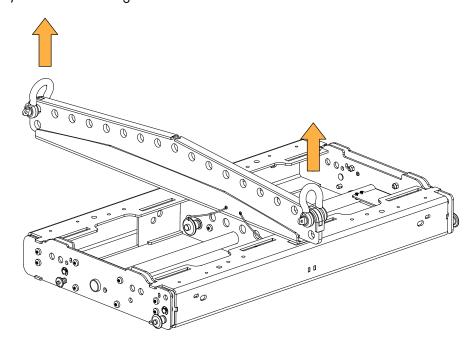
**3.** Lower K3-BUMP to facilitate the connection between the enclosures and the rigging frame.
