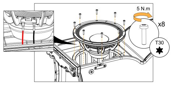
If the speaker gasket is damaged, remove and replace it.
