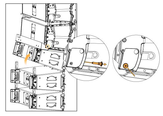
b) Secure the front KARA-DOWNK3 tabs to the K3 rigging. Slightly lower the K3 array if necessary.
