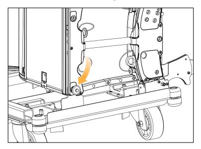
**4.** Lift the rear of the enclosure and rotate the dolly rear rigging arm in its upward position.
