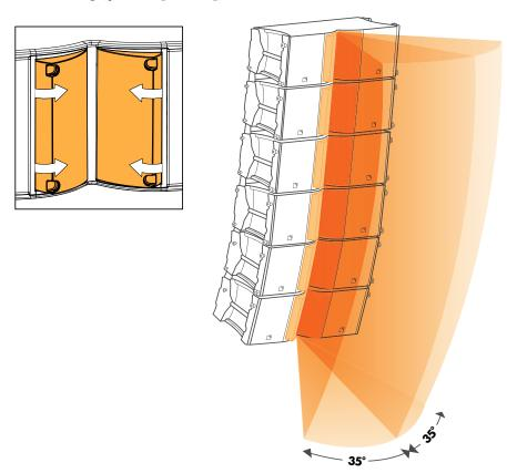
Set the fins in the 70° position to provide the system with a 2 dB on-axis gain (> 1 kHz), compared to the 110° setting.
