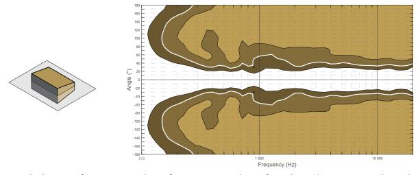
Dispersion angle diagram of a K3 array with  $70^{\circ}$  fins setting, using lines of equal sound pressure at -3 dB, -6 dB, -12 dB.
