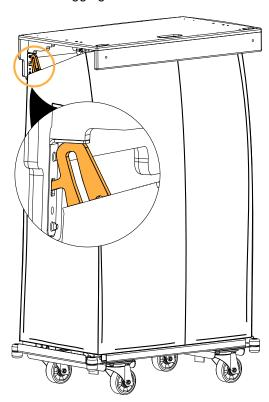
**5.** Connect the front rigging arms of K3 Secure the ball-locking pin to the front rigging arm.
