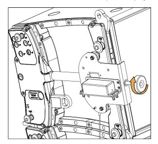
5. Secure the K2-LASERMOUNT by running the sling inside and around the K3 handle and locking it on itself.
