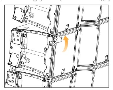
b) Secure the front rigging arm to the LINK of the flown array with the ball-locking pin.
