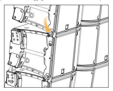
c) Lower the flown array and secure the assembly with the LINK pin.
