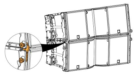
• The front rigging arms can be deployed with some resistance, and rotate correctly.
