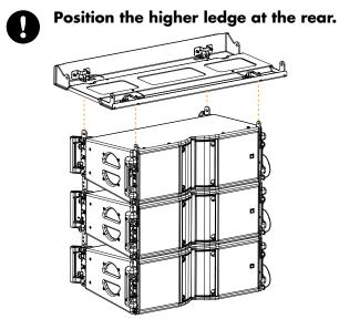
Secure the Kara II rigging arms inside the slits with the ball-locking pins.
