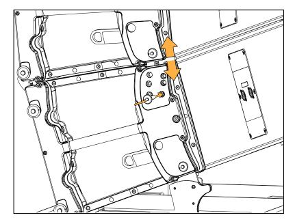
**3.** Press the lock button to lock the inter-enclosure angle.
