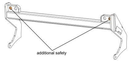
K3-RIGBAR is equipped with two shackles to secure LA-SLING2T.
