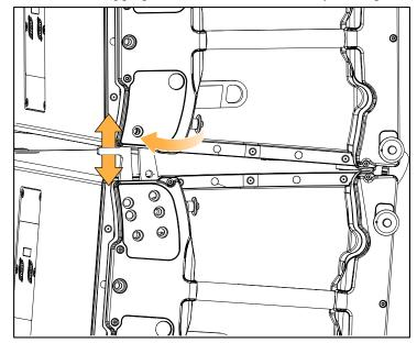
d) Secure the chosen angle with the ball locking pin.
