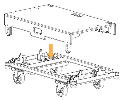
2. Secure K3-CHARIOTLID to the front rigging arms of K3-CHARIOT using the locking pin.
