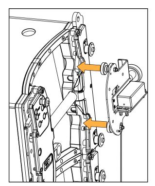
$\textbf{4.} \ \ \text{Maintain the K2-LASERMOUNT in position by tightening the knob.}$
