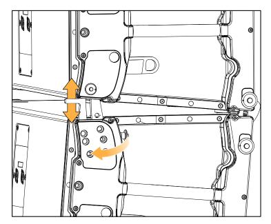
e) Press the button to activate the automatic locking system.
