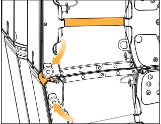
**8.** Slide the rear rigging arm and secure it with both pins, in the LINK and  $10^{\circ}$  holes.
