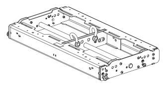
Four holes are available on the central bar of K3-BUMP for site angle adjustments. Four additional holes are available to add K3-BAR to K3-BUMP as an extension to increase the site angle.
