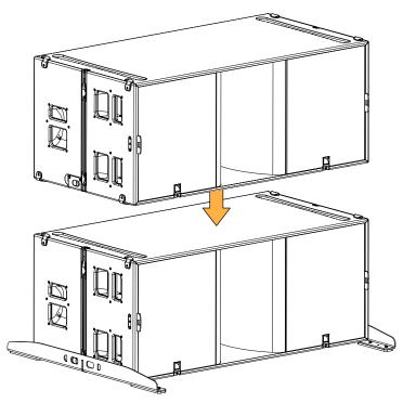
Connect each enclosure on both sides before adding the new one.
