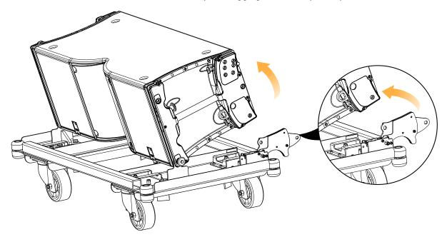
**5.** Secure the enclosure using the LINK hole.
