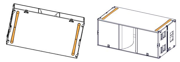
KS28 features eight L-shaped side runners for side protection and upright stacking.
