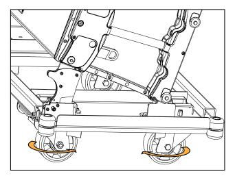
b) Pull back the bottom enclosures while lowering the array until the array and the top enclosure of the second block are in contact.
