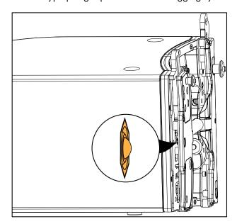
**4.** Secure the rear rigging arms at one of the inter-enclosure holes.
