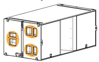
KS28 features two ground runners for enclosure protection. Two tracks on the top of the enclosure fit the ground runners in stacking deployment.
