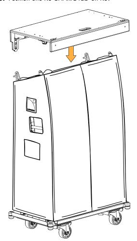
**4.** Position the back of K3-CHARIOTLID on the rear rigging arms. The rear rigging arm must be in the notch of K3-CHARIOTLID.
