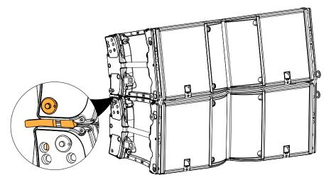
• The rear rigging arms can be deployed with some resistance, and slide correctly.
