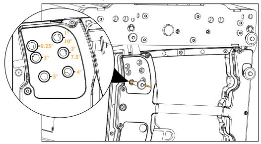
**5.** Raise the array to lock the inter-enclosure angles.
