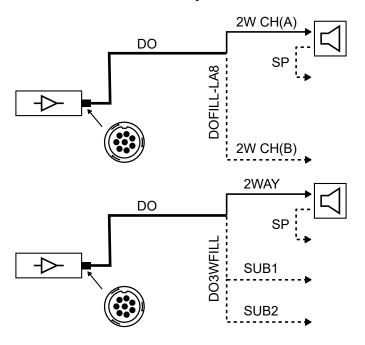
b LA8 can drive up to two KS21 or KS21i per output, but no more than six per controller at high level.
