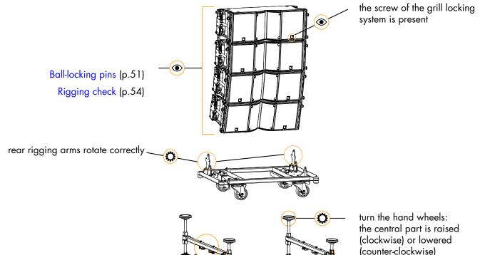
the locking handles can be tightened and loosened by hand
