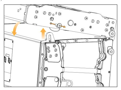
d) Attach the rear rigging arm to the frame.
