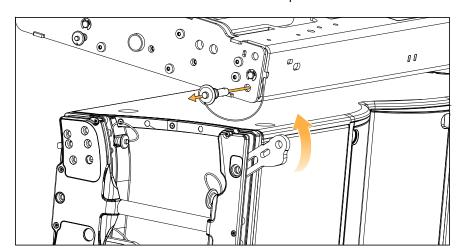
b) Lower the K3-BUMP and secure the connection with the K3 pin. If the pin resists, move the frame back and forth.
