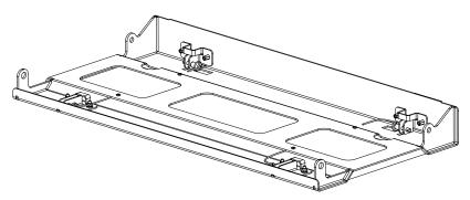
The four tabs on the top are compatible with the  ${\rm K3}$  rigging system.
