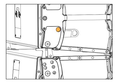
**4.** Raise the array to lock the inter-enclosure angles.
