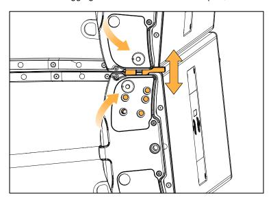
**9.** Make sure the automatic locking system button is unloaded. If the button has been pressed, pull to disengage the latch.
