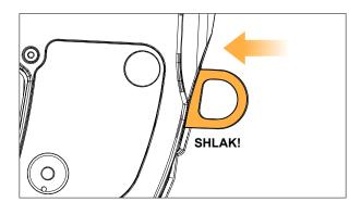
**7.** Disassemble the two enclosures.
