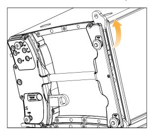
**3.** Position the K2-LASERMOUNT on the side of the enclosure.
