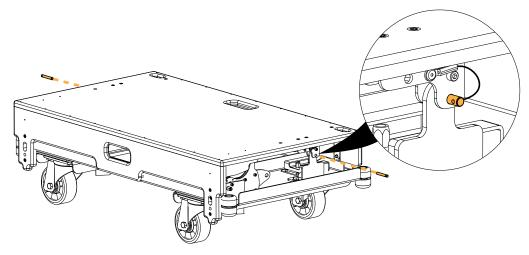
**3.** Position another K3-CHARIOTLID (reverted) on the first one. The longer side must be on the front side of K3-CHARIOT.
