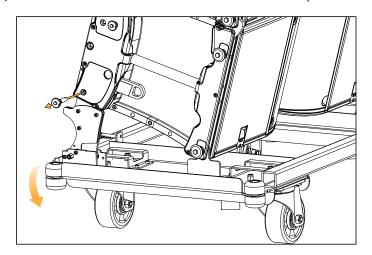
b) Hold the chariot with one hand. Remove the front pin on both sides.
