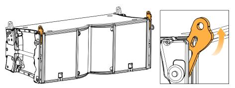
• The ball-type plunger protrudes out the rigging system.
