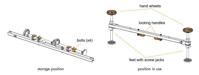
With K2-JACK, the site angle of the K3 array can be adjusted between -23° and +13°.
