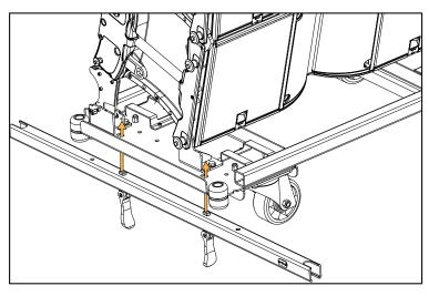
b) Raise and turn the K2-JACK handles to secure the locking system.
