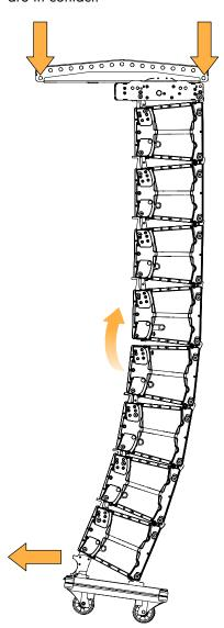
c) Slide the rear rigging arm and secure it with the pin using the LINK hole.
