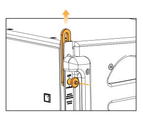
b) Slide up the rear rigging arms and select the same inter-element angle, from 0° to 10°.
