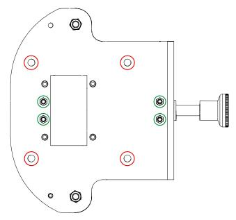
To mount the LAP-TEQ PLUS / LAP-TEQ / RECLINE, use the bracket delivered with the inclinometer.
