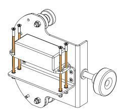
It is also possible use the LASER-MAGPLATE associated with the LAP-TEQ PLUS or LAP-TEQ. In this case, the inclinometer must be calibrated for a vertical use.
