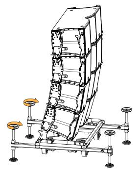
With the front screw jacks for a positive site angle.
