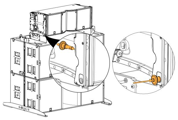
b) Secure the rear arms of K3-TILT to the bottom rear of the enclosure. Connect the K3 ball-locking pin to the rear sliding arms of K3-TILT.
