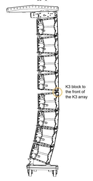
a) Rotate the front rigging arm to align its hole with the K3 rigging hole.
