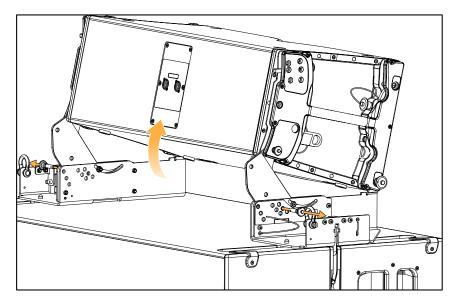
Set the angle and secure the sliding arm with the ball-locking pin.
