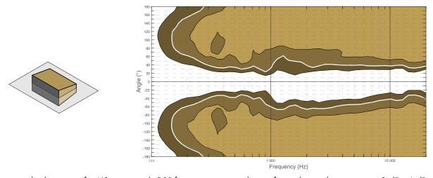
Dispersion angle diagram of a K3 array with 90° fins setting, using lines of equal sound pressure at -3 dB, -6 dB, -12 dB.
