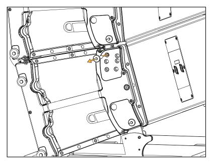
2. Position the pin at the chosen angle hole and slide the rigging arm until the pin goes in.
