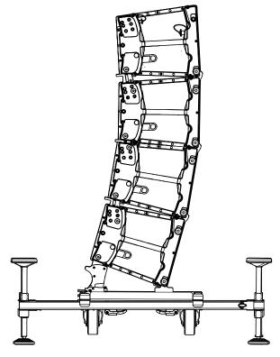
2. Loosen one stabilizer bolt and tighten the other one depending of the target site angle.
