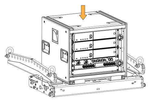
**5.** Secure the LA-RAK II AVB with the coupling bars.
