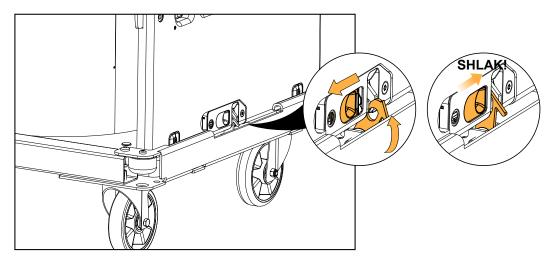
4. Disconnect a stack from the array on both sides.
