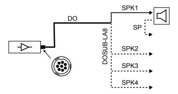
For passive loudspeakers, the value corresponds to the number of enclosures in parallel on the output. For active loudspeakers, the value corresponds to the number of sections in parallel on the output.
