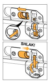
2. Secure A15-BUMP or A15-RIGBAR on top of the array.
