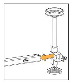
Insert the feet at both ends of the bar.
