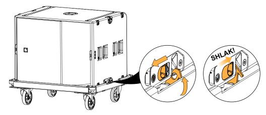
**3.** Secure another KS21 on the assembly. Align the runners with the tracks.
