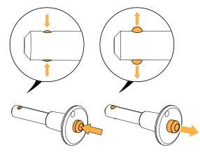
**3.** Insert the pin in each storage and rigging hole. Pull and rotate the pin. The pin must remain inside the hole.
