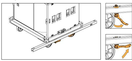
2. On each K2-JACK foot, rotate the wheel counter-clockwise until the central part is close to the base.
