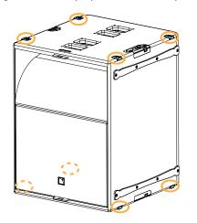
The logo on the enclosure front can be rotated to adapt to every configuration.
