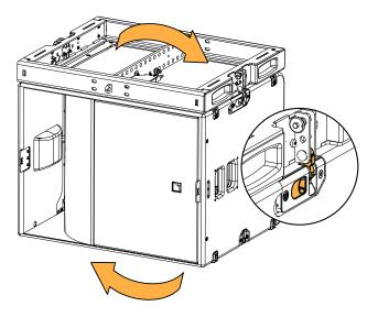
The rigging arms are fitted with yellow safety labels, that are visible when the rigging arm is not in use.
