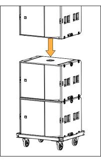
b) Connect the enclosures on both sides.
