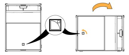
KS21 features a 35 mm pole-socket which contains an M20×150 insert.
