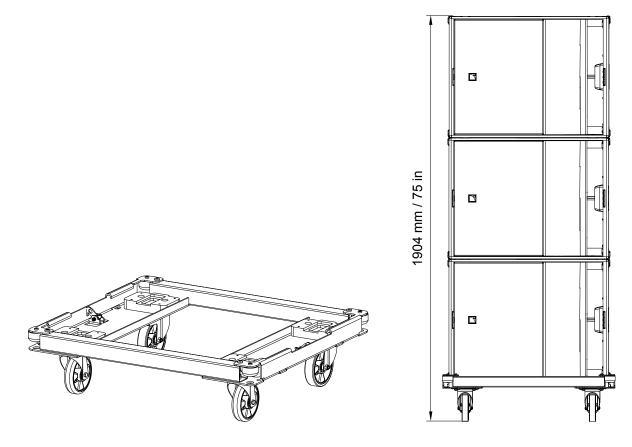
KS21-CHARIOT features two brakes for optimal stability.
