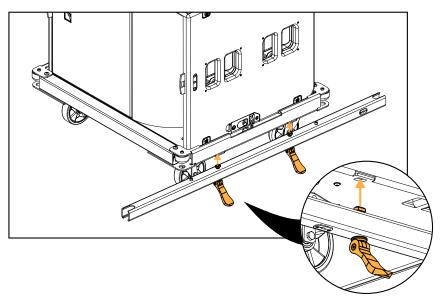
b) Raise and turn the locking handles to secure the bars.
