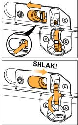
The rigging elements are fitted with yellow safety labels that are visible when they are not safely locked.
