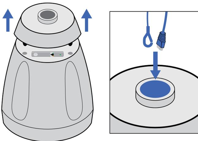
4. Clip the suspension cable's hook to the loudspeaker and plug in the Ethernet cable.
