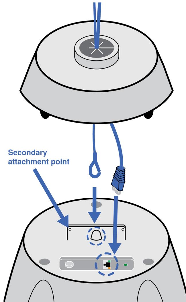
5. Press the back cover onto the loudspeaker.
