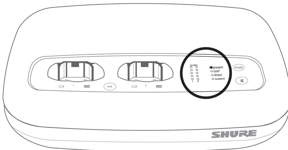
3. Place the microphones in the docking bays of the APXD2. When docked successfully, the microphones will turn on, and the battery LEDs on the APXD2 will illuminate. The microphone displays will also show the charging status.
