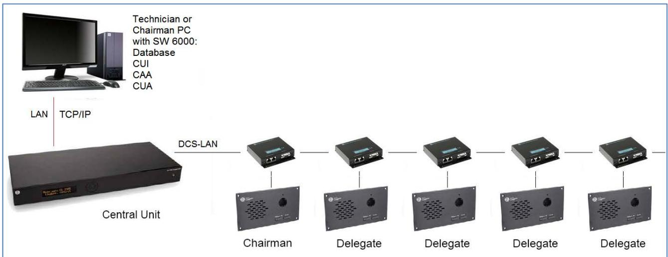
Figure 3.2-A Standard one PC installation
