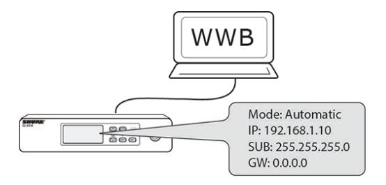
3. Compare the IP address assigned to the component to the available IP addresses listed in to the *Network Selection* window. Choose the network that closely matches the numbering order and format of the IP address of the component (192.168.1 in this example). Select *Save* to finish.
