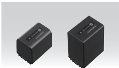
NP-FV70A (7.3 V / 13.8 Wh / 1900 mAh) NP-FV100A (7.4 V / 25.9 Wh / 3410 mAh) Rechargeable Battery Pack
