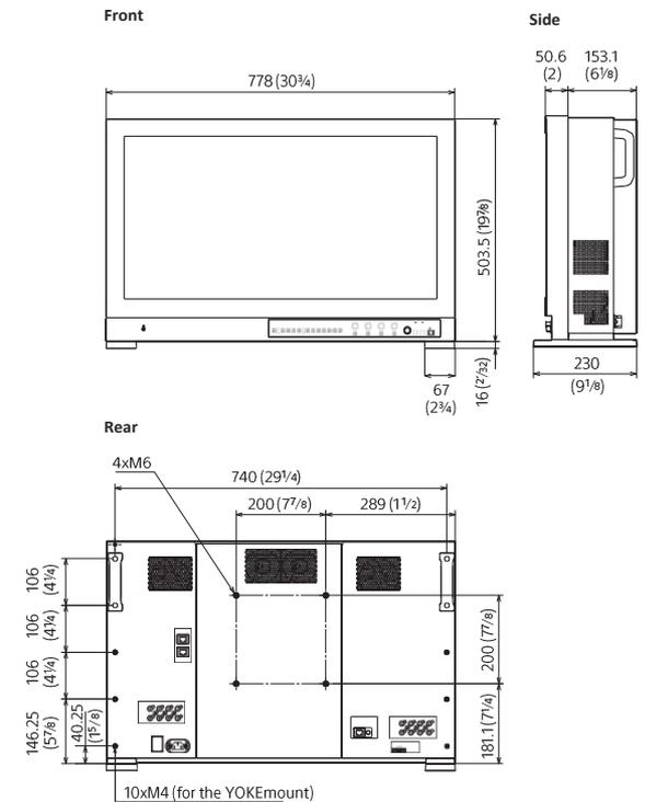
To install on a vehicle, fix the unit using screw holes for the YOKE mount.
