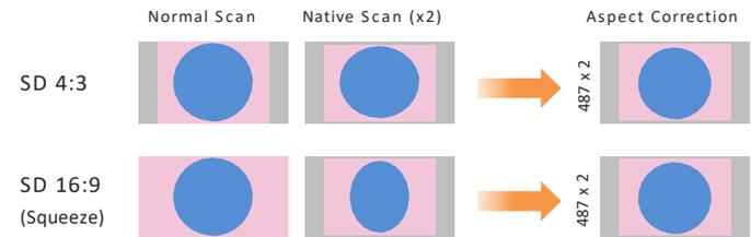
Example of NTSC signal on the 16:9 aspect panel – BVM-E250A
