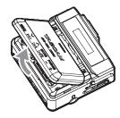
**2.** Install 2 AAA batteries with their  $\oplus$  and  $\ominus$  marks as shown in the battery compartment, and close the cover.
