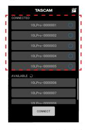
Example with 5 devices added to the list When a device is added to the CONNECTED list, it will begin connection standby and connection will automatically be attempted.
