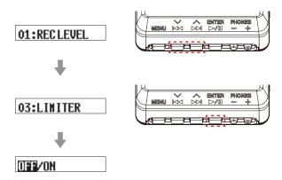
**3.** Use the  $\bowtie$  [ $\backsim$ ] and  $\triangleright$  [ $\backsim$ ] buttons to change the setting value/item.
