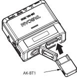
Insert the connector toward the unit's display.
